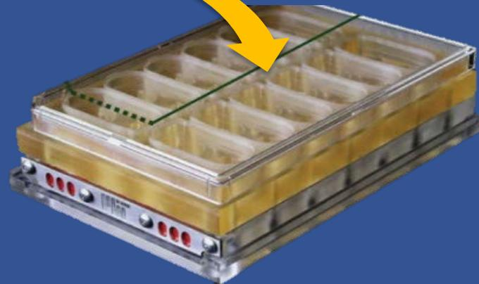
12-well microfluidic bioreactor plate (LiverChip)
